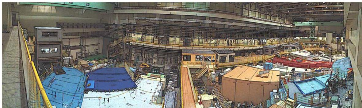
**Figure 1.** Artistic panoramic view into an experimental hall of the Materials and Life Science Facility at J-PARC [2–5]. The neutron beam ports surrounding the target station are to the far right feeding beamlines at the right, while muon apparatus is located in the left side of the image.
